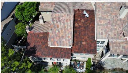
Association has installed composite roofing material on one roof of a residence on Emerald Downs Drive. The two areas replaced each had more than 50 golf ball impacted broken clay roof tiles and were selected candidate areas as prototype composite а roofing material. The Association's roofing engineer investigating the builder's roofing construction and installation defects recommended the composite material for its durability and aesthetic appeal. The material is commonly
